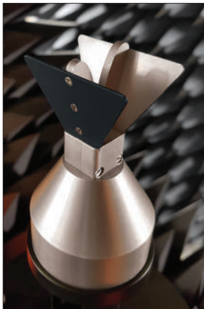
▲ Fig. 1 The SH 4000 dual ridge horn antenna, used as a test case for the StarLab 50 GHz.
