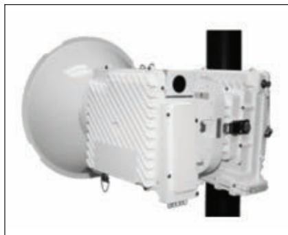
▲ Fig. 1 One end of a typical 2+0 XPIC point-to-point microwave radio link with traditional single-carrier transceivers that provides 1 Gbps data rates.
